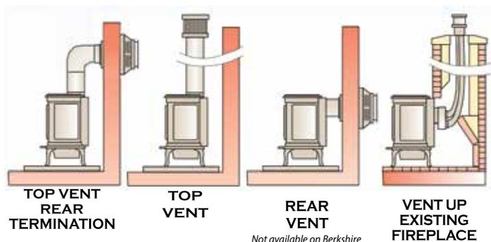
Rear Vent Installation - Lopi gas stoves have a rear vent installation option to make installing your unit as quick and easy as possible. The Minimum Rear Vent Kit is designed to give your stove optimum performance. Included in the Minimum Rear Vent Kit are: Flue adapter, 3.9" section, wall thimble, wall thimble cover, and a horizontal cap. This comes with everything you need to install your gas stove in the most cost-effective way. Talk to you Lopi dealer about this option.
