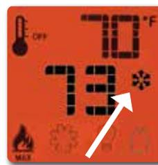
Use Continuous Pilot during the fall and winter months or in cold climate areas where more heat is desired. This mode keeps the Pilot on at all times and warms the vent system to maintain a strong draft in the chimney and reduce moisture condensation on the glass.
