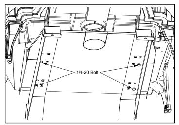
Figure 5.1 - Remove unit from shipping brackets.
