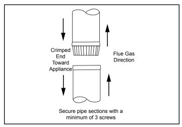
Figure 4.6 - Chimney Connector (Appliance Pipe)
