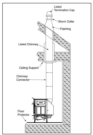
Figure 4.2 - Prefabricated Interior Chimney
