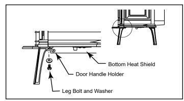
Figure 5.4 - Handle holder and heat shield positions.
