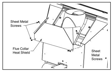
Figure 5.6 - Install flue collar heat shield.
