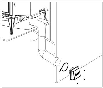
Figure 5.13 - Floor Installation
