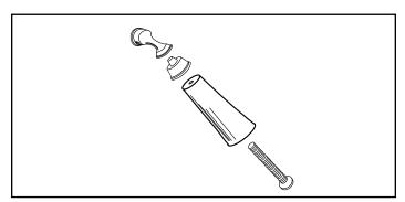
Figure 5.3 - Assemble the front door handle.
