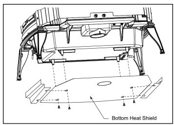
Figure 5.5 - Attach the bottom heat shield.
