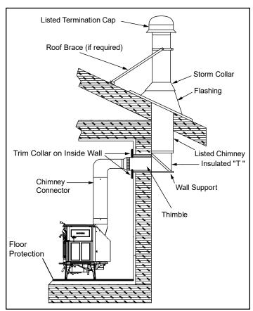
Figure 4.1 - Prefabricated Exterior Chimney
