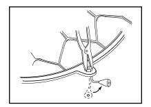
Figure 5.2 - Attach the griddle handle.
