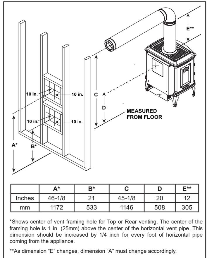
Figure 5.2 - Wall Penetration
