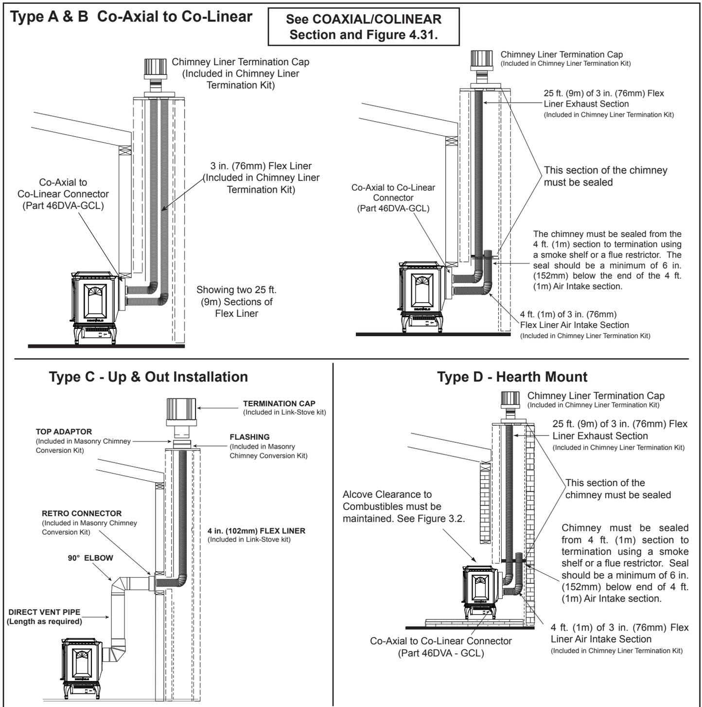
1. Before cutting any holes, assemble the desired sections of direct vent pipe to determine the center of the masonry penetration.
