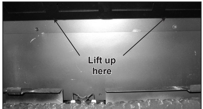
Figure 6.10 - Remove Upper Baffle
