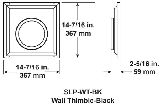
Figure 11.2 - SLP Series Vent Components
