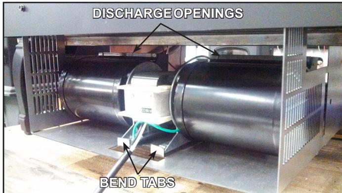
Figure 8.4 - Fan Housing
