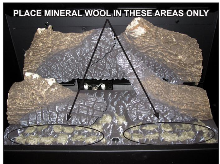
Figure 5 - Placement of Mineral Wool
