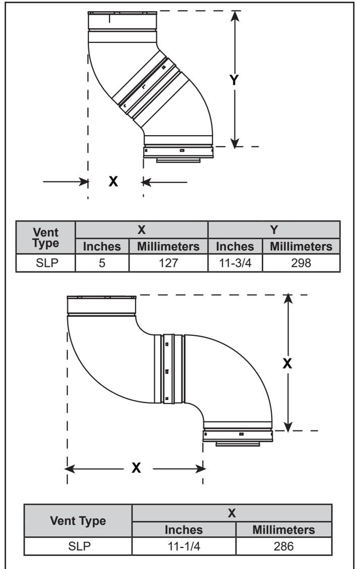
Figure 4.5 - Vertical and Horizontal Offset for SLP Elbows
