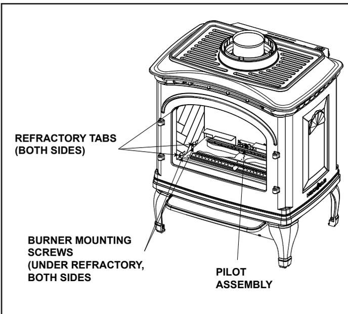
Figure 6.13 - Remove Burner
