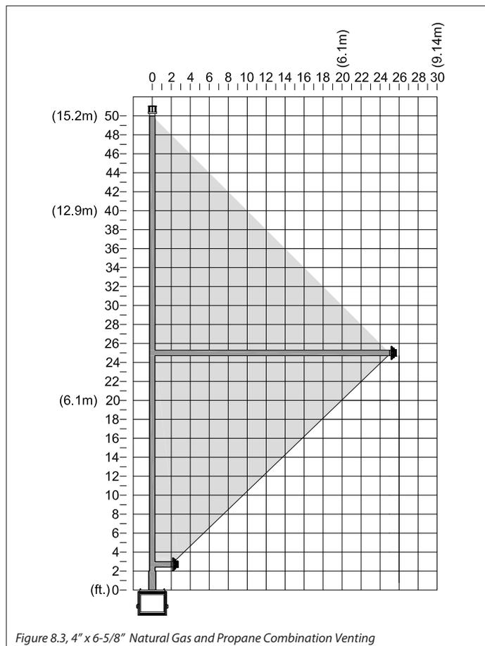
Figure 8.3, 4" x 6-5/8" Natural Gas and Propane Combination Venting
