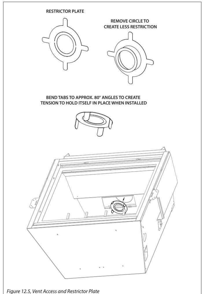
Figure 12.5, Vent Access and Restrictor Plate
