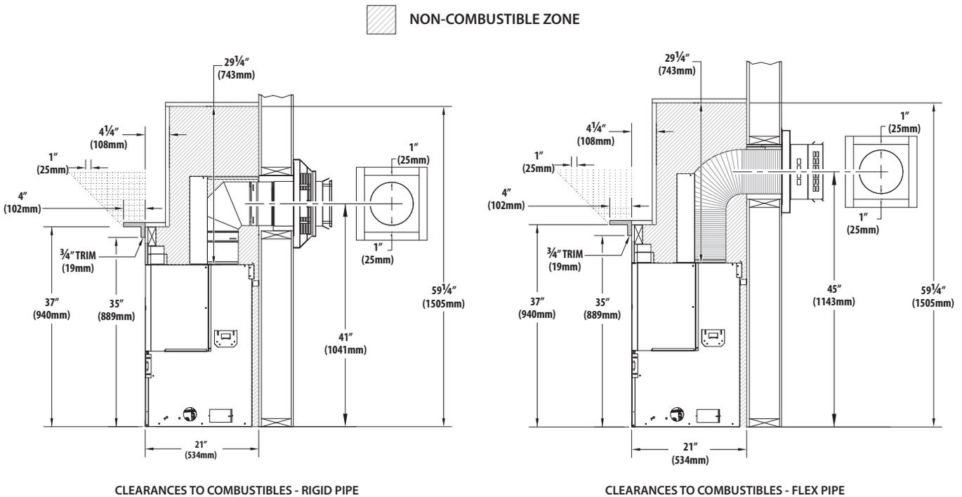
Figure 3.1, Clearance to Combustibles
