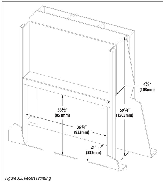
Figure 3.3, Recess Framing
