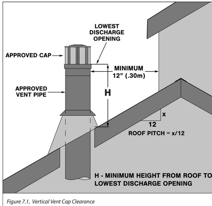
Figure 7.1, Vertical Vent Cap Clearance
