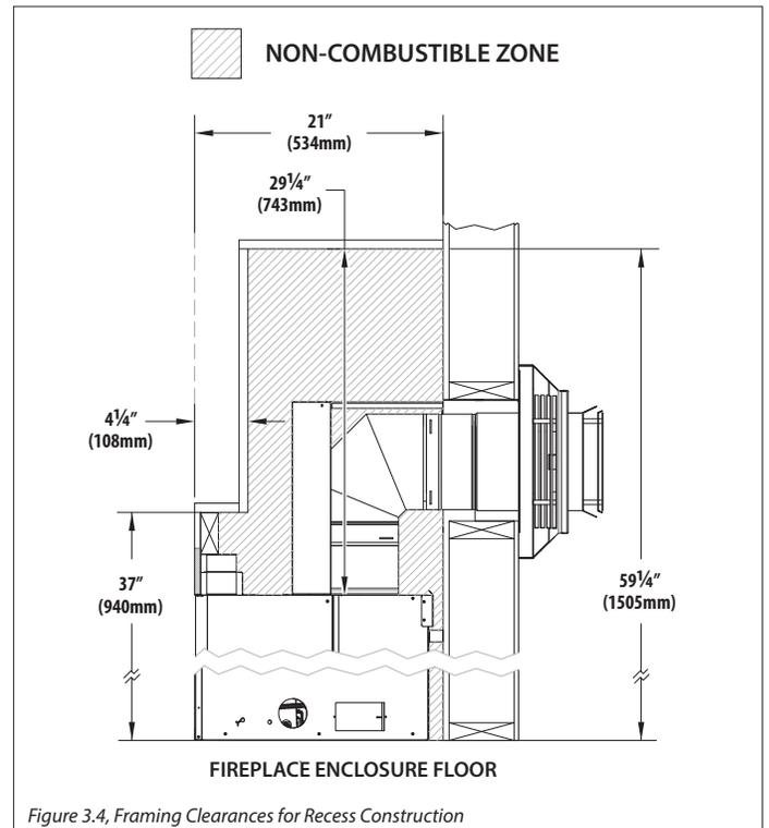
Figure 3.4, Framing Clearances for Recess Construction
