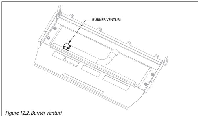
Figure 12.2, Burner Venturi
