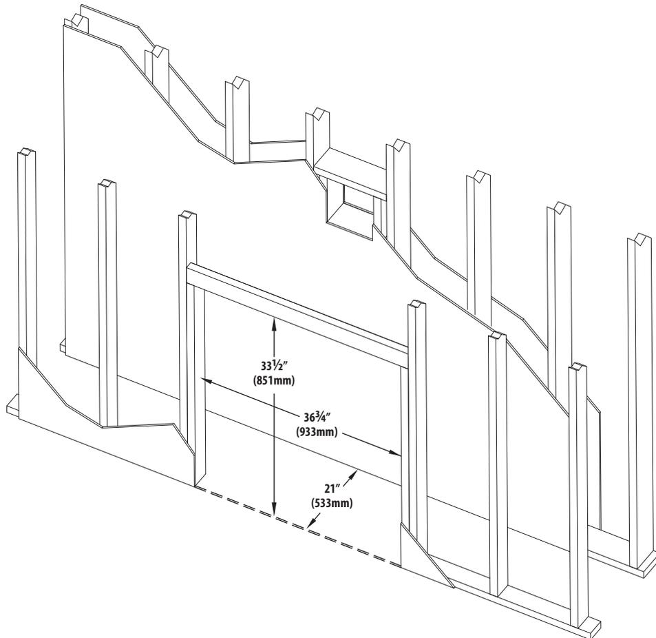
Figure 3.2, Framing Dimensions
