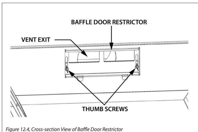
Figure 12.4, Cross-section View of Baffle Door Restrictor
