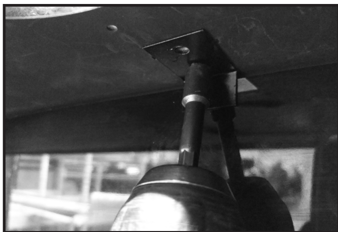
Figure 3 Retaining Bracket Installation - Back
