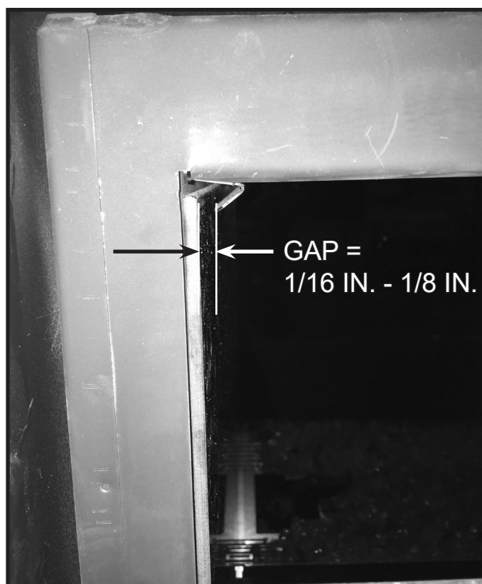
Figure 6 Gap Between Tab and Side Glass Panel: 1/16 IN. - 1/8 IN.
