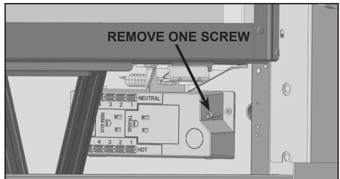
Figure 8.3 Junction Box Detail - COSMO32-IFT-B
