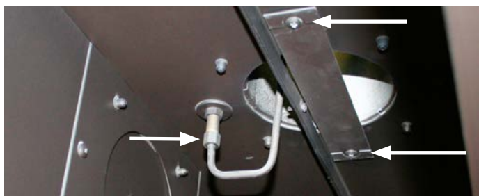
Figure 5.c Removal of Top Vent air baffle and pressure sensing tube
