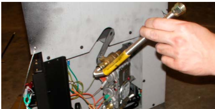
Figure 4.3 Converting the gas regulator on the valve
