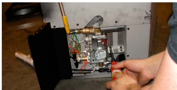
Figure 4.2 Propane conversion kit showing pilot orifice, main burner orifice,
